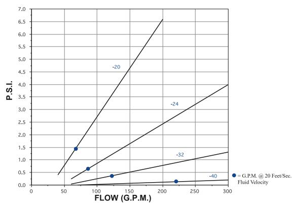
Tests conducted with 150 SUS oil at 100°F with Female Pipe (FP) X Female Pipe (FP)
